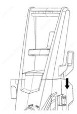
3. Installing the spray wand. Fit the spray wand into the gun and rotate it until the two parts are completely locked.
