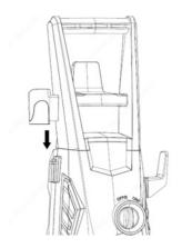
2. Slide the power cord hook into position of unit left.
